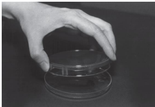
Figure 4: Opening a petri plate culture. The bottom is lifted out of the top, and the top is left lying face up on the bench.
